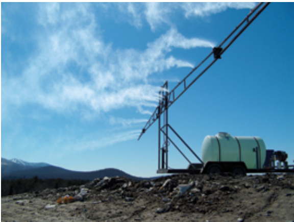
Photo: NCM Odor Control This portable system features nozzles at 5-foot intervals.
